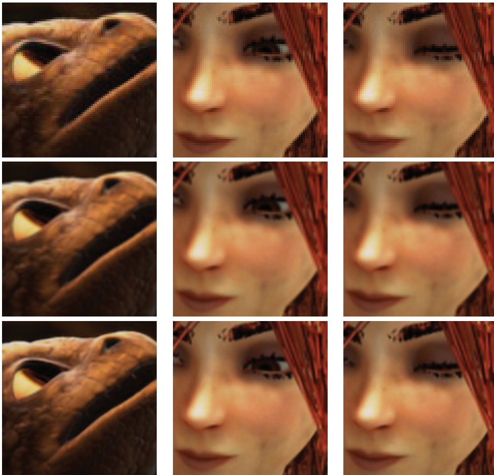
Figure 4. Single-image SR estimates for data set #1. Details of the SR images obtained with nearest neighbor strategy (first row), Lanczos interpolation (second row), and the learning algorithm proposed in [41] (third row).
