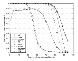
Figure 1: Frequency of exact reconstruction versus number of nonzero coefficients; N = 128, M = 256,  $\sigma_w^2 = 10^{-5}$ ,  $\sigma_r^2 = 10$ .
